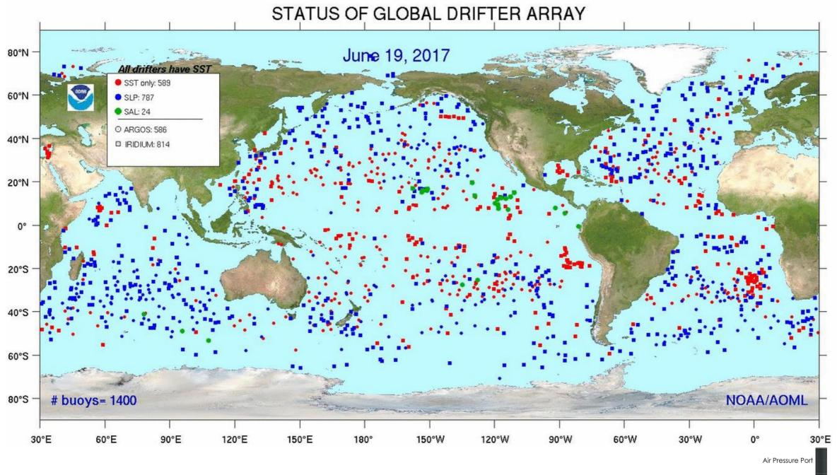
The NOAA funded GDP is a global array array of surface drifters that measure **Essential Climate Variables, including** near-surface ocean currents (15 m depth), sea surface temperature, sea surface salinity, sea-level air pressure, and directional wave spectra.
